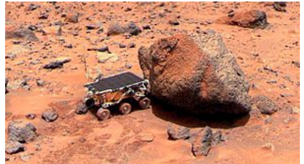
Sojourner takes Alpha Proton X-ray Spectrometer measurements of the Yogi Rock .
